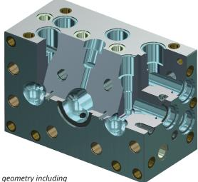
Automatically identify complex hole geometry including intersecting and non-conventional holes.
