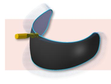
**Curve 5-axis:** This toolpath is one of Mastercam's oldest and most popular. The cut pattern follows a curve (a line, a spline, a circle, or a surface edge) that can be wireframe, solid,or surface.
