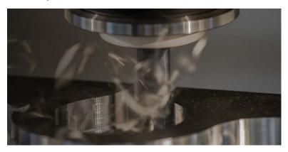
These 2D and 3D high speed dynamic milling toolpaths utilize the entire flute length of their cutting tools to achieve great efficiency in milling. They are designed to maximize material removal while minimizing tool wear.
