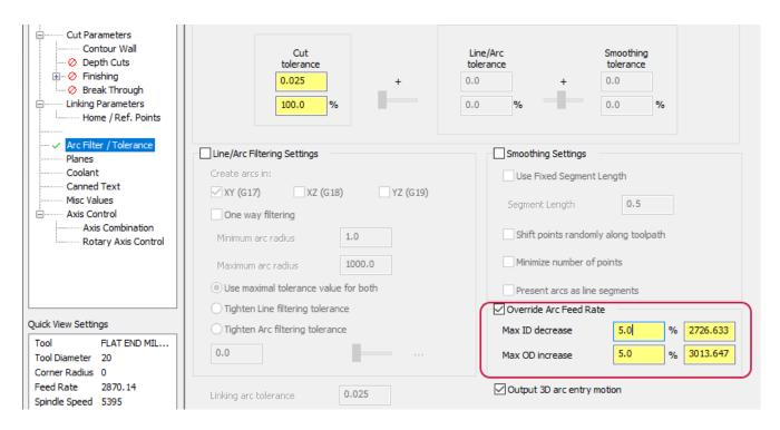
Override Arc Feed Rate increases and decreases the arc feed rate when cutting around corners. The base feed rate is set on the Tool page.
