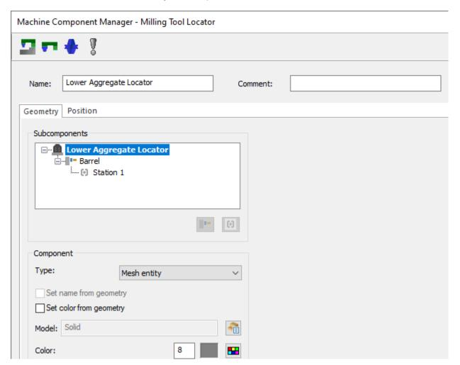
Milling tool locators can include a barrel subcomponent. This represents the portion of the locator that rotates, and typically is associated with its own solid model. A barrel is optional; you do not need to include one if it is not necessary. In the picture below, the orange model is the barrel subcomponent.
