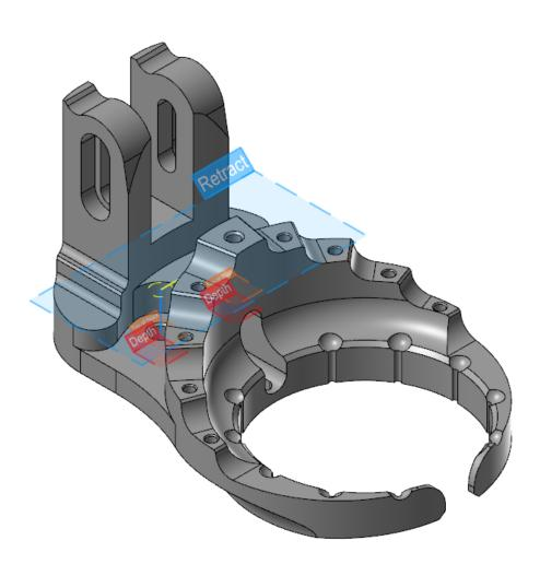
When you change values in the dialog box, Mastercam updates the graphical planes in the graphics window. You can also change the position and value of a plane by dragging its graphical representation in the graphics window, as shown in the following image. During this dragging, you can type a value into the box that appears with the gnomon. Additionally, you can drag the plane indicator to an AutoCursor point.
