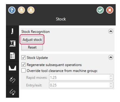
When you click the button, Mastercam displays the existing remaining stock model relative to the chained geometry in a temporary viewsheet. A green ball indicates the beginning of the chain, and a red ball indicates the end. The gray dashed line indicates the current stock boundary.
