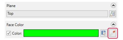
If you cannot easily select the face color in the graphics window, you can also click **Select color** to choose a color from the **Colors** dialog box. Mastercam continues to disassemble the part placing the largest, flattest face of a body towards the layout plane. However, it will also place any face of this color that is the same size of its opposing face towards the layout plane.
