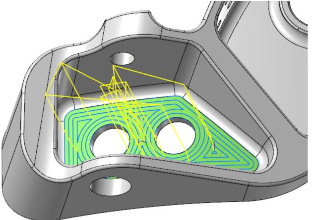
The display of colors for selected geometry is controlled by the **Display graphical elements** button in the dialog box's toolbar. To hide the colors, turn off the **Display graphical elements** button. This button is on by default.
