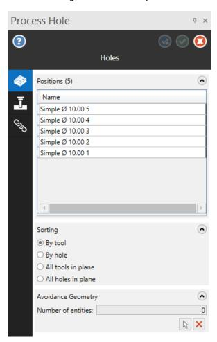
The operations library controls tool type and number, feeds and speeds, and operation order. The Process Hole operation determines geometry selection and linking parameters. You can use both 3- and 5-axis scenarios for Process Hole geometry selection. At any point after creating a Process Hole operation, you can explode the operation into its component operations and work directly with those components like any other toolpath.
