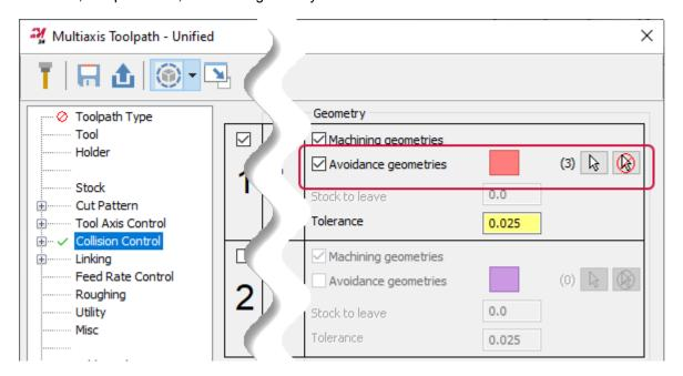
The same type of counter is available in the **Toolpath Hole Definition** panel for hole making toolpaths. This counter shows the number of features selected for holes and is handy when the number of selected features is greater than can fit in the list.
