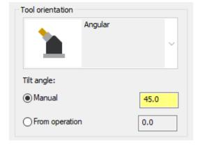
Angled heads can be created with a fixed angle, or you can configure them to get the angular orientation from the operation. This affects how you set the toolplane.
