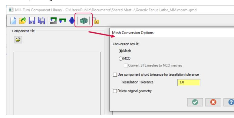
You can choose between two desired output formats: Mesh or MCO. Mesh converts the solids to Mastercam mesh entities. MCO converts the solids to an encrypted mesh format.
