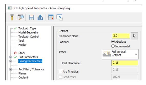
The actual retract height is set by the **Clearance plane**. However, if the retract height is less than the **Part clearance**, Mastercam adds an additional linear move between them until the total height equals the **Part clearance**.
