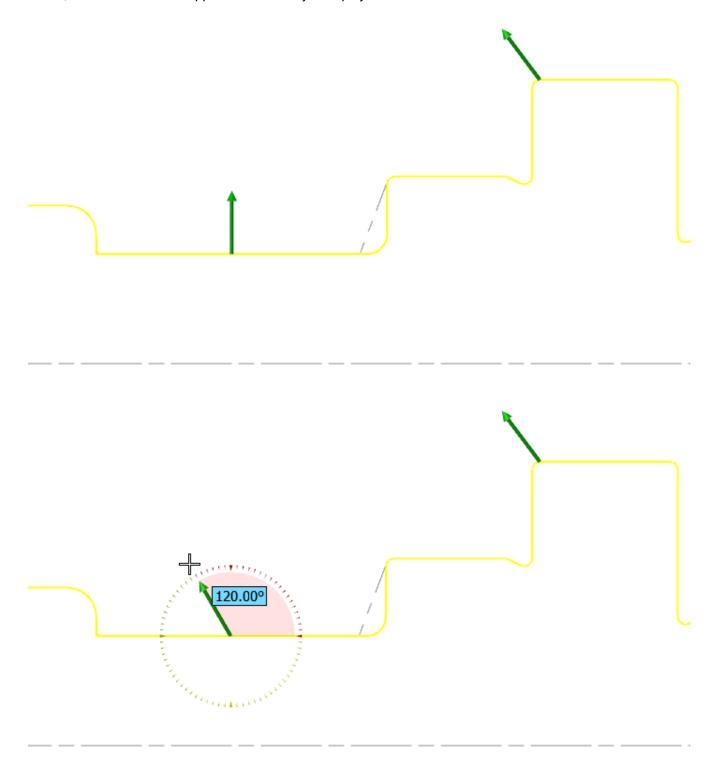
Double-click anywhere on the contour to add additional tool axis vectors. Sections of the contour, where the tool is not able to contact the part, are highlighted in red; if you double-click in a non-contact area, Mastercam will add the new tool axis vector at the closest possible location.
