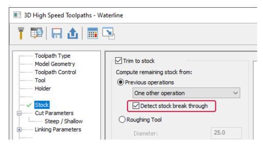
Use the **Detect stock break through** option to eliminate air cuts where no stock is below the previous pass. This option is only available when **Previous operations** is set to **One other operation** and the operation is a stock model.
