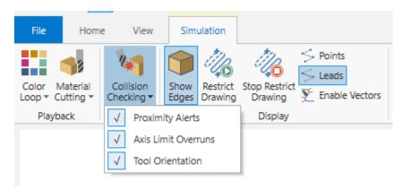
You can also select **Tool Orientation** as a **Stop Condition**, which is set on the **Home** tab. When selected, Mastercam Simulator pauses your simulation when a tool insert does not match the spindle direction.
