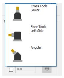
Angled heads can be locked to a fixed angle (select **Manual** and enter the angle), or can be set so that the angular orientation comes from the operation. Other new properties include a **Speed multiplier** factor plus the ability to **Reverse spindle direction**; these should be set to match the internal gearing on your head.
