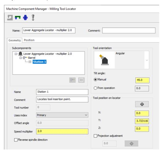
Milling tool locators can be oriented for face milling, cross milling, or angular. Face- and cross-milling tool locators support multiple stations per locator, while angled heads allow only one.
