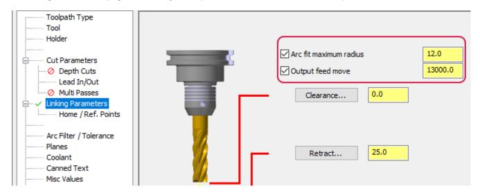
**Arc fit maximum radius** attempts to fit 90-degree arc moves into rapid and clearance moves. If the entered radius does not fit, then the output creates a 180-degree arc.
