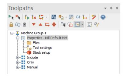
Instead, Mastercam Simulator now only uses the information in the **Machine Group Setup** panel to populate the simulation. Options previously found in the **Simulation** and **Data** tabs of **Simulator Options** are found in the **Simulation** page.
