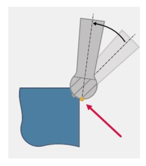
Use this option to prevent the possibility of additional burrs when cutting, such burrs sometimes occurring due to the zero SFM at the tip of the tool. You can find **Avoid contact point on tip** in the **Tool Axis Control** page for Deburr toolpaths.
