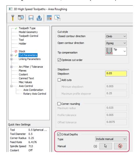
Choose the **Type**, which determines the type of flat area to be machined by a single Area Roughing contour. Choose between the following:
