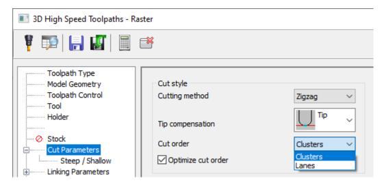
Lanes cut the part in one direction. Clusters finishes a section before moving to the next.
