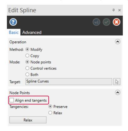
When you select the **Align end tangents** option in the panel, Mastercam matches the tangency of the repositioned spline endpoint to that of the destination endpoint. The blended geometry results in a continuous curvature of the geometry and a better foundation for surface creation.
