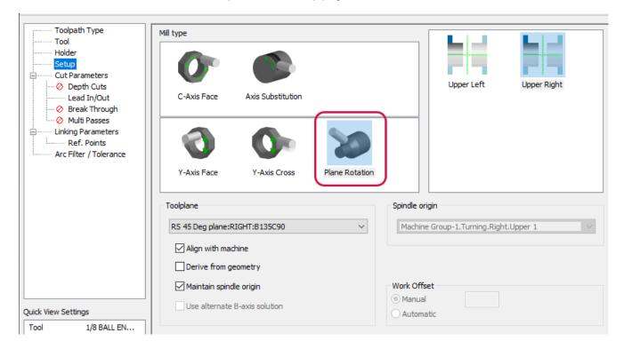
Typically this setup type is not available for turret-only machines, but will be required whenever the milling head is oriented at any angle other than 0 or 90 degrees. The orientation of the head also filters the allowable axis combinations.
