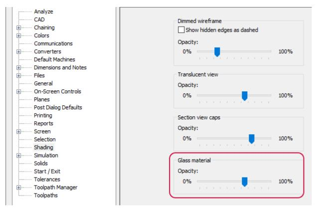
Additionally, in **Outline Shaded** mode, adjustments to the opacity of a translucent entity now affect the entity edges. In previous versions of Mastercam, the opacity setting affected the translucency of the entity but did not affect its edges. The examples below are set to **Glass level 4**.
