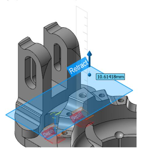
By turning off the **Display plane labels** option in the **Display graphical elements** drop-down, you can remove the labels from the plane indicators, leaving you with a simpler display. When the labels are off, you can hover your mouse pointer over a plane to see its label.
