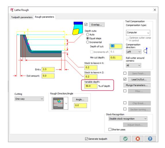
The adjustment is applied to alternate passes, meaning that your cutting passes will alternate between straight and angled cuts. However, in flat areas, a straight cut will be made instead of an angled cut. If the cut length is less than the cut depth, a straight cut will be made instead of an angled cut.
