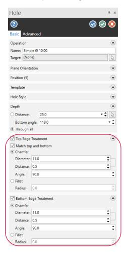
While in previous versions of Mastercam, you could only create a chamfer at the top edge of a hole, Mastercam 2024's new **Top Edge Treatment** parameters allow you to create either chamfers or fillets on your hole edge. Mastercam has also expanded options to generate a chamfer by giving you the option to specify the size of the chamfer by entering either its diameter or its width distance.
