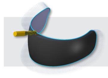
**Curve 5-axis:** This toolpath is one of Mastercam's most popular. The cut pattern follows a curve (a line, a spline, a circle, or a surface edge) that can be wireframe, solid, or surface.
