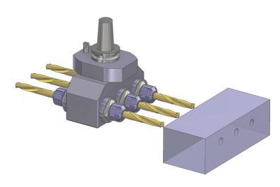
Mastercam Router streamlines multiple tool programming including block drills and aggregate heads.
